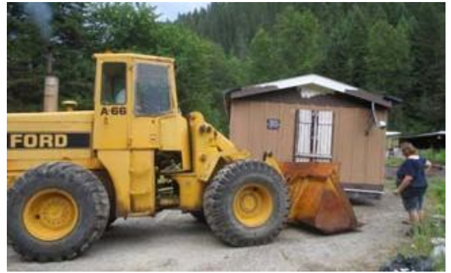
Using a hitching ball set in the bucket of his backhoe, John Hopper is able to move Krista Kirby's trailer (manufactured home) to where the old trailer was parked.
